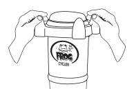
Replace cap by hand only. DO NOT OVER TIGHTEN.
