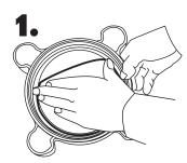
Hold cap in front of you upside down with the o-ring groove facing up. Place one end of o-ring into cap groove at the point closest to you. Hold o-ring down with the thumb and index finger of one hand.
