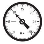
Check the pool's filter gauge often and periodically clean filter per the manufacturer's directions. A dirty filter will slow the flow of water which could hamper proper circulation.
