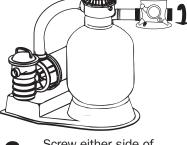
Screw either side of POOL FROG® Cycler on to open nipple end until upright and secure.
